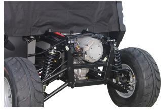
**Front differential** - Featuring Electric Differential Lock System. Simply push the button on the dash control that is exposed when the vehicle is in 4WD mode and the front differential locks so that both front wheels are in drive mode.
